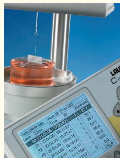
Measuring of the surface tension with Wilhelmy plate
